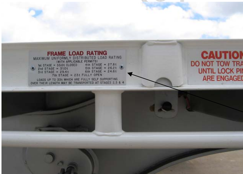
Photo 5. Typical Frame Load Rating Plate located on roadside coaming.
