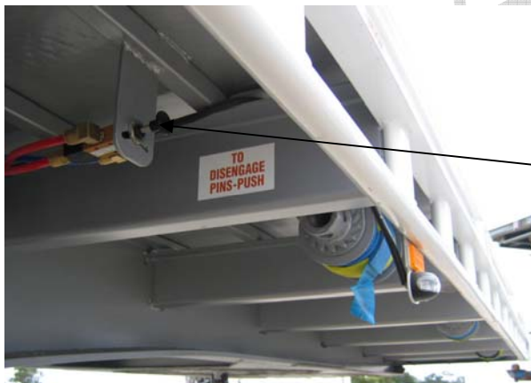
Photo 2 Air valve – Push to disengage pins, Pull to engage pins
