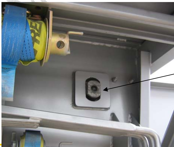
Photo 3 Locking pin engaged – protrudes through locating hole
