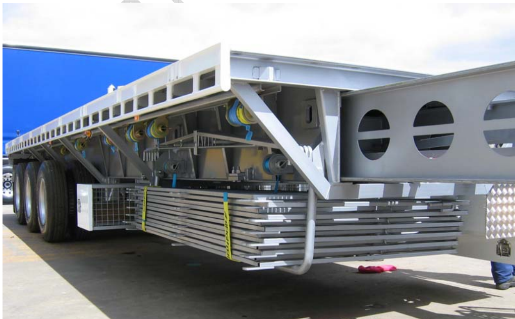
Photo 1. General view showing sliding main rails arrangement
