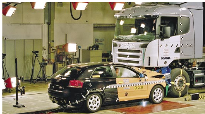
Truck collision Testing of Front Underrun Protection
