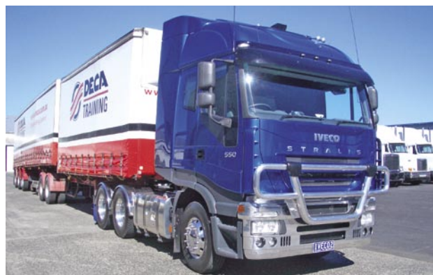
Example of a complying 26 metre B-Double — Cab Strength, Front Underrun Protection, compatible bullbar & 20.6 m trailer set.
